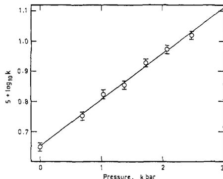
Figure 1. Pressure dependence of the first-order rate coefficient  $k$  ( $\text{sec}^{-1}$ ) for the exchange of all six waters of  $\text{Cr}(\text{H}_2\text{O})_6^{3+}$ ; the error bars represent  $\pm 3\%$  uncertainty in  $k$ .
